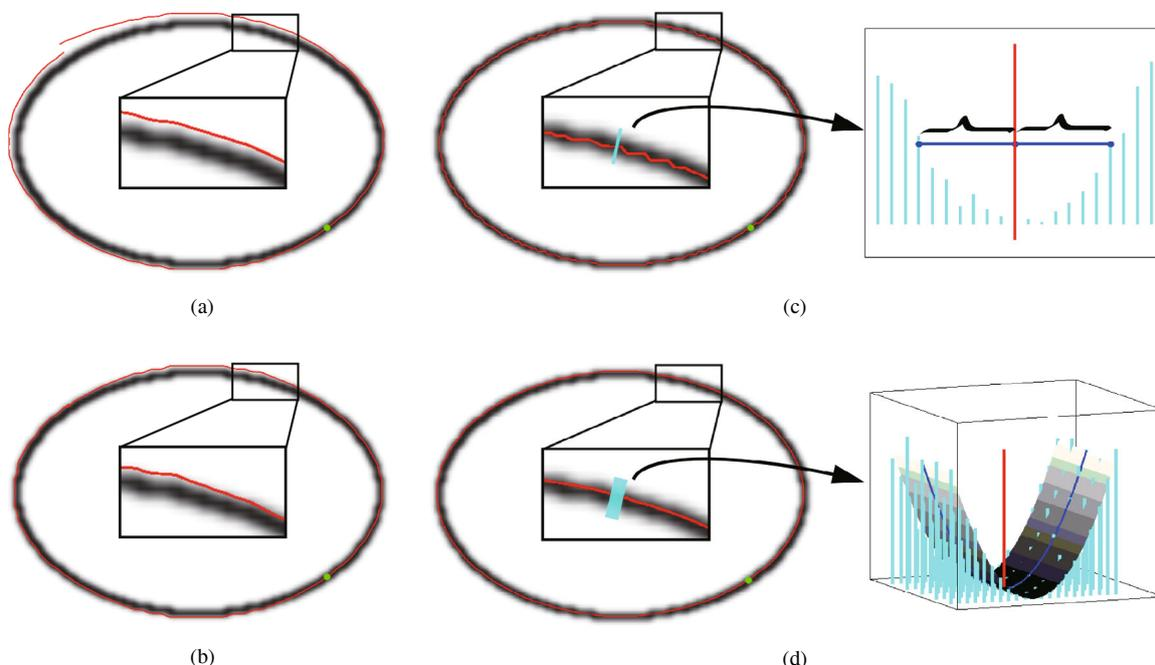
**Figure 2** (a) Euler method; (b) Runge-Kutta method; (c) central point correction; (d) our fitting-based correction. To illustrate our improvement on line tracking accuracy, we take an elliptic without junctions as an input image. The tracking starts from the green point and ends until both sides meet. In (c) and (d), heights of the blue lines indicate luminance in local sampling neighborhood, red lines in the middle represents the correcting tracking position (under Frenet frame).
