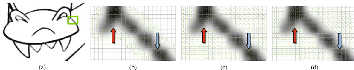
**Figure 1** (a) Input image; (b) Sobel filter; (c) first-order Gaussian derivative; (d) our method. Vector field computed using Sobel filter has a poor smoothness (b); the one computed using first-order Gaussian derivative (with a standard variance 1) is smoother, but over-smooths at junctions (c); our tensor-based method overcomes these shortcomings (d). Note that we use green bar to illustrate the normalized vector of each pixel.
