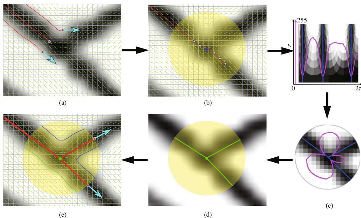
**Figure 5** Pipeline of junction analysis: a junction is detected by directional difference through contour tracking on both sides (a); then we take even-spaced samples on the central tracking path to get potential junction centers (b); a luminance polar mapping technique (c) is employed to analyze both branch number and their orientations simultaneously (d); finally, topological structure is determined by the smoothness of contour paths (e).
