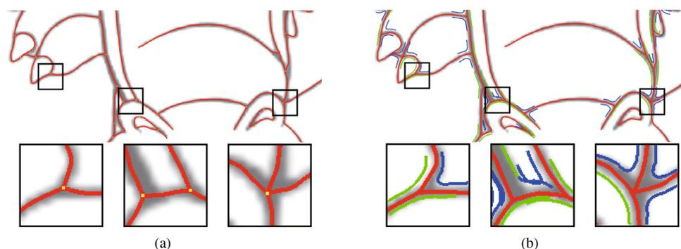
**Figure 7** Intermediate results for junction analysis. (a) Junction centers and branch numbers; (b) smoothness between adjacent branches. Our method reconstructs lines in junction regions according to the smoothness of contours (b), it improves the one only using branch numbers (a). Note that green curves are  $G^1$  continuous, and blue curves are not  $G^1$  continuous.
