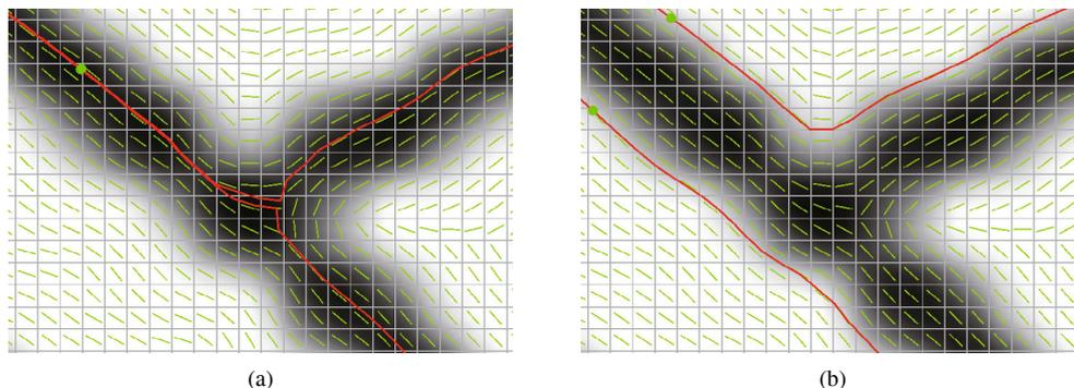
**Figure 4** Comparison the stability between midpoint tracking and contour tracking. (a) Starting from two midpoints whose distance is only 0.1 pixel separately, two tracked lines diverge each other around junctions, it shows central line tracking is very sensitive; while contour tracking is rather stable and accurate as in (b).
