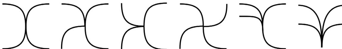
**Figure 3** Examples for junctions with four branches. Different topological connection (i.e. smoothness) brings a big challenge for the vectorization task around junctions.
